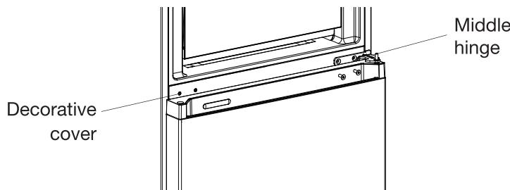
3. Remove the freezer door ( be careful not to lose small parts such as the shaft sleeve and stop on the door ).
