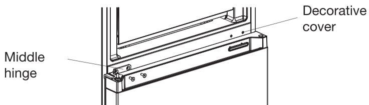
7. Install the refrigerator door on the middle hinge and install the upper left hinge.
