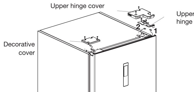
2. Remove the fridge door ( be careful not to lose small parts such as the shaft sleeve and stop on the door ).
