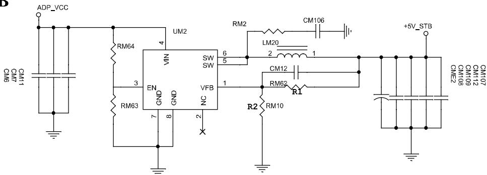
$$V_{out} = 1 + R_1/R_2 = 5.1V$$
