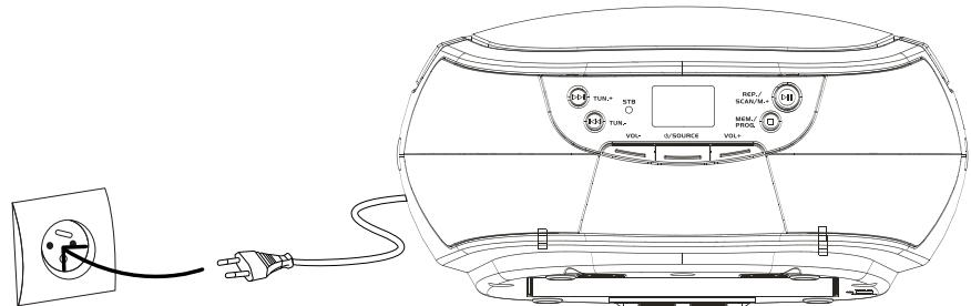
Plug one end of the power cord into the power connector on the back of the radio. Then plug the other end into a mains outlet. The red power light comes on.
