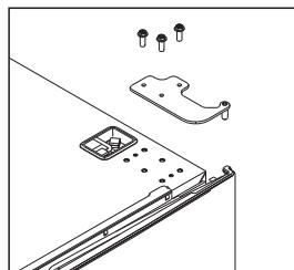
6. Unscrew the screws in the top-left hinge cover and remove the cover.
