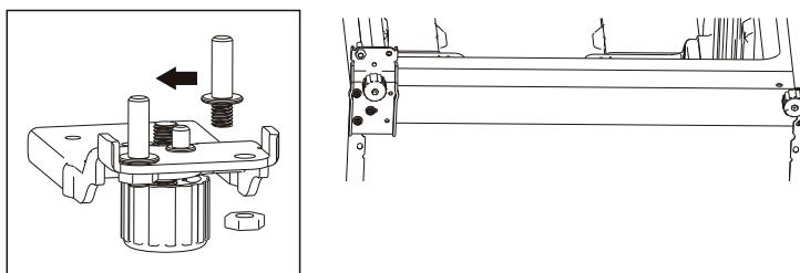
15. Reinstall the adjustable feet. If necessary, adjust the adjustable feet to make the refrigerator level.
