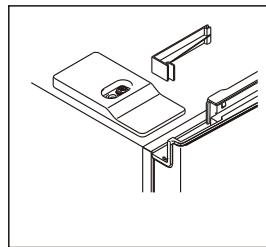
4. Unscrew the two screws on the top-right hinge cover. To do this, loosen the screws with a socket wrench and then use a crosshead screwdriver to remove them.
