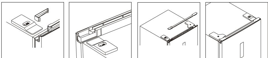
13. Reinstall the hinge cover onto the right side over the screw holes. Remove the tape from the grey screw hole cover (that can be found in the accessory bag) and press the grey cover firmly over the exposed screw hole.
