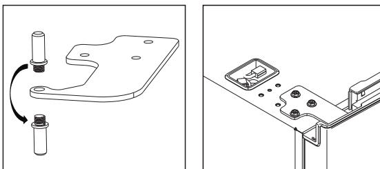
10. Remove the door switch from the top-right hinge cover by pressing the bottom of the switch upwards and then install it in the top-left hinge cover which can be found in the accessory bag.
