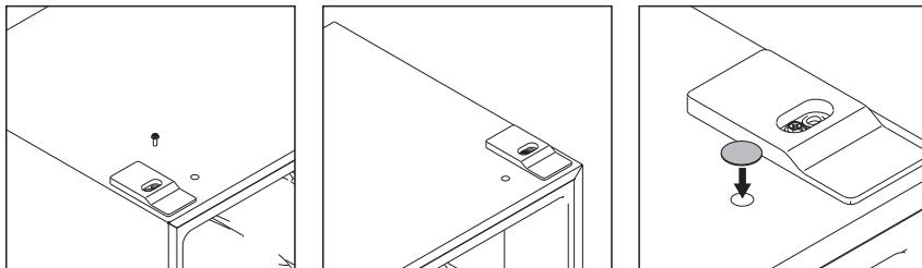
14. Using an adjustable wrench, unscrew and move the hinge pin on the bottom hinge to the adjacent hinge pin hole. Place the hinge over the top-right hinge screw holes and fix into place with the three hinge screws. Tighten the screws using the socket wrench.
