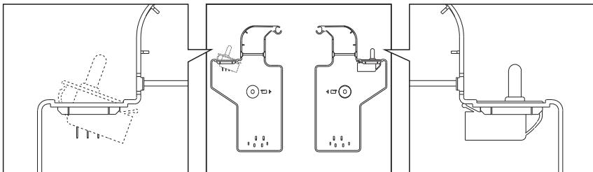
11. Connect the door switch and the display screen wire connectors and then slot the wires into the clips inside the hinge cover. Take a look at the photo you took earlier to assist you with this step. Fix the left-hinge cover into place.
