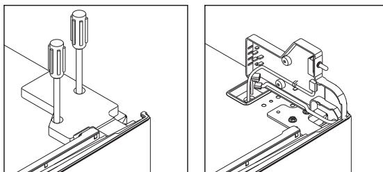
5. Unscrew the top-right hinge. To do this, loosen the three screws with a socket wrench and then use a crosshead screwdriver to remove them.
