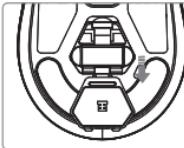
Remove the USB receiver from the compartment and insert it into a free USB port on your computer.
