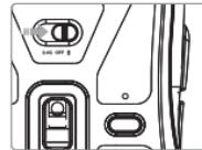
Slide the mode selector switch to position . Briefly press the pairing button to select the bluetooth channel\*: the indicator light turns green for the **BT1** channel or blue for the **BT2** channel.
