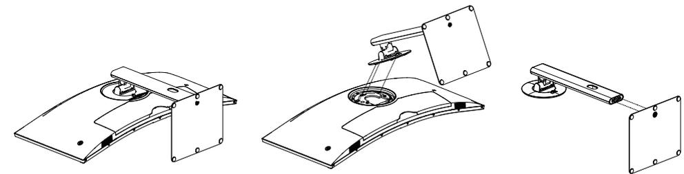
To remove the stand, pull the locking latch at the back of the screen upwards, then tilt the screen forward before lifting it.
