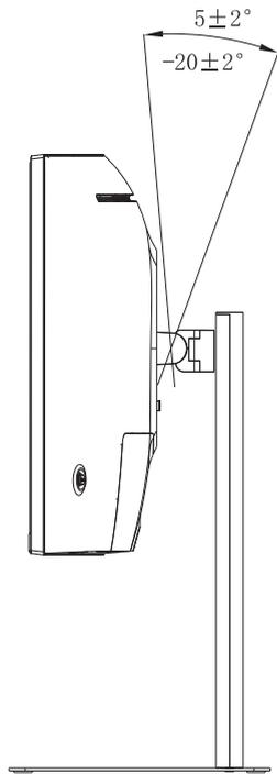
Note: when adjusting the screen angle, hold the screen stand with one hand and adjust the tilt with the other. Using both hands prevents the screen from falling.
