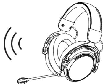
If you have a Bluetooth\* audio device (smartphone, tablet, laptop computer, etc.), wireless connection allows you to listen to music played on your audio device without using a cable. To benefit from the play/pause function, make sure your device (mobile phone, audio player, etc.) is compatible with the A2DP and AVRCP Bluetooth\* profiles.
