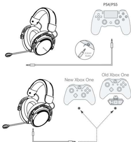
To use the headset in wired headset mode with the supplied 3.5 mm audio cable:
