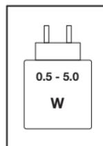
The power delivered by the charger must be between min 0.5 Watts required by the radio equipment, and max 5.0 Watts in order to achieve the maximum charging speed.
