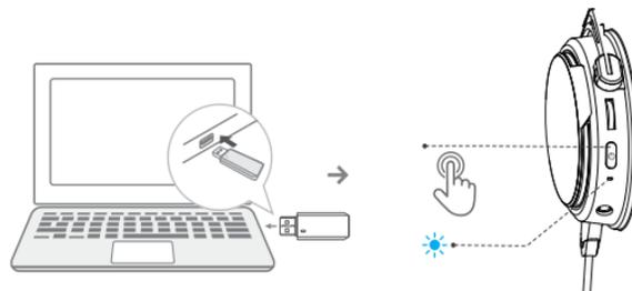
1. Plug the adapter into a free USB port on your computer. The indicator light on the wireless adapter flashes blue, indicating that it is waiting for a connection.
