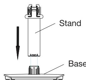
2. Lay the monitor down flat on a flat, stable surface covered with a soft cloth, then slide the stand into the notch until you hear a click. To remove the stand, press the coded pins, then pull the stand downwards.
