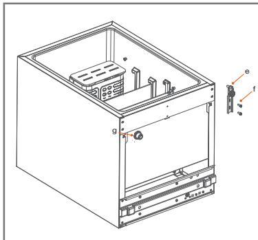
5. Place the lower hinge (e) on the opposite side and screw in the screw (f). Then position the adjustable foot (g) on the opposite side.
