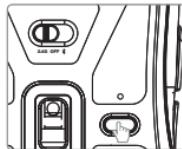
Press and hold the pairing button for 3 seconds. The indicator light flashes quickly.
