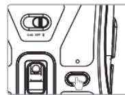
Press and hold the pairing button for 3 seconds. The indicator light flashes quickly
