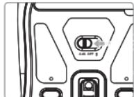
Slide the mode selector switch to the **2.4G** position. The indicator light turns red.
