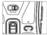
Press and hold the pairing button for 3 seconds. The indicator light flashes quickly.
