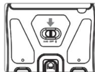
Slide the mode selector switch to the **OFF** position. The indicator light goes off.
