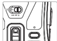
Slide the mode selector switch to position . Briefly press the pairing button to select the bluetooth channel\*: the indicator light turns green for the **BT1** channel or blue for the **BT2** channel.
