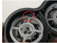
Make sure that the notches on the plastic circle are correctly positioned over the notches on the removable cradle, then clamp the two sides together.
