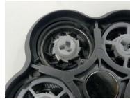
The blade and protective grille can then be removed.
