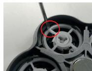
To clean the heads, start by unclipping the plastic ring with a screwdriver, applying pressure between the plane and the head support.
