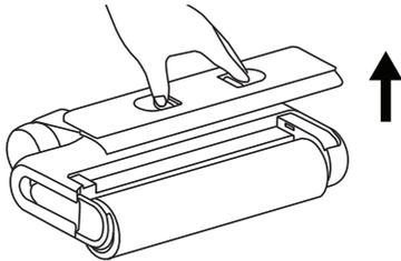
2. Align the roller brush cover with the floor brush, press it down, and the roller brush cover is installed when a clicking sound is heard.
