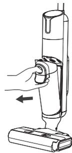
2. Hold the tank body with one hand and pull out the dirty water tank upwards with the other hand.
