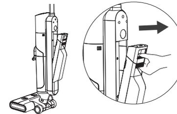
6. First put the bottom of the clean water tank into the opening position on the back of the cleaner body, gently push the clean water tank, and the clean water tank is installed when you hear a clicking sound.
