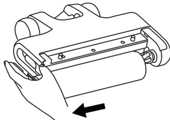
2. Align the right end of the roller brush with the right end of the floor brush, push it to the right, and insert the left handle into the corresponding position. At the moment, the roller brush is installed.
