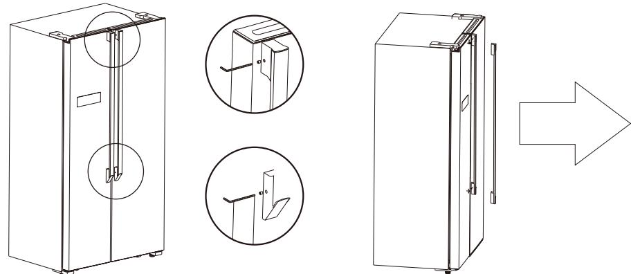
If the doors in your home are not wide enough to move the refrigerator, you can remove the two door handles: Unscrew the handles with an allen key, then pull the handles out. Proceed in reverse order to attach both handles back to the refrigerator.
