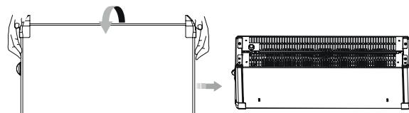
4. Position and secure each foot on each side of the appliance using the screws provided.
