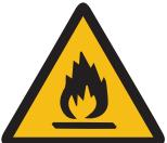
This “Danger symbol; fire hazard/flammable materials” symbol indicates that the refrigerant gas in your appliance is flammable in the event of a leak resulting from damage.
