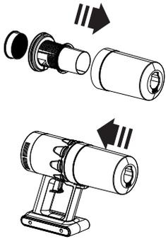
B. Hold the host and press the disassembly dust cup component in the opposite direction. Align the reference point of unlocking dust cup on the dust cup with the reference point of the host.
