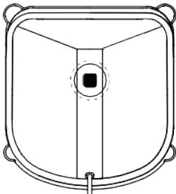
After placing the device on the glass, the blue light will flash slowly for a few seconds until it reaches the suction necessary to start the movement safely. Once the blue light is solid, the user can press a button on the handle or a button on the remote control to start cleaning.
