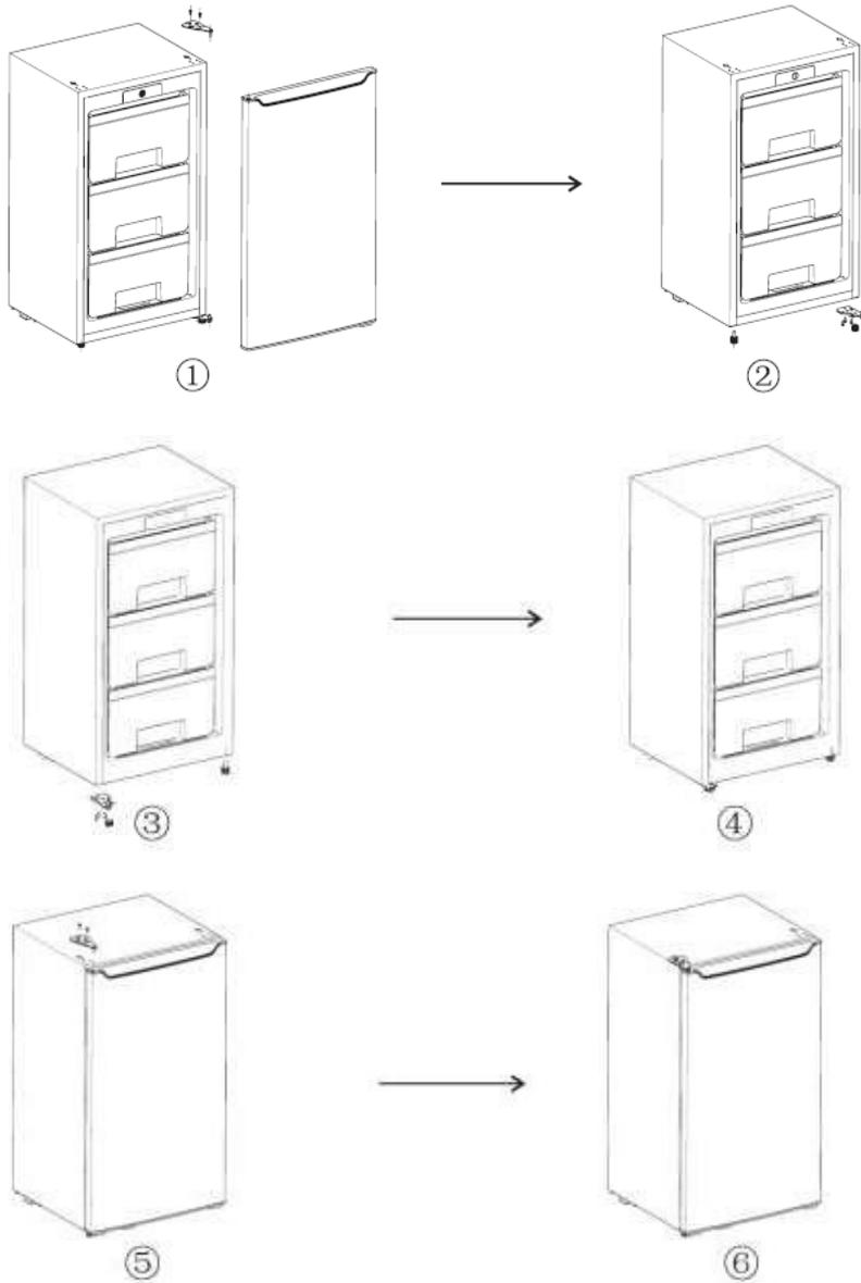
1. Remove the two screws of the upper hinge. Remove the top hinge and disassemble the door. Set it aside carefully.
