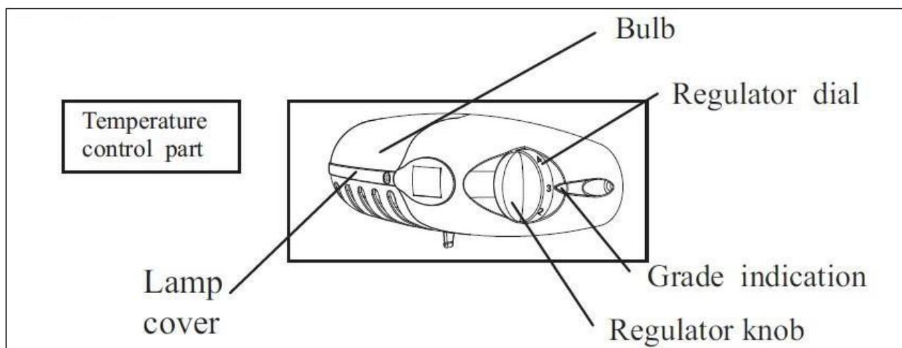
Your refrigerator has one control for regulating the temperature. The temperature control is located on the lower right-hand corner.
