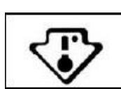
You will find the symbol opposite in your refrigerator. It clearly shows the location of your appliance's coldest zone: the temperature here is + 4°C or less. A temperature indicator here enables you to check that your refrigerator is working correctly.
