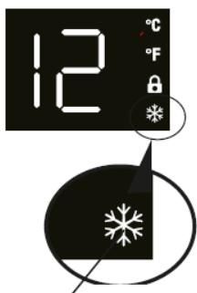
When the compressor is running, a warning light is displayed and remains visible; the indicator will be off when the compressor stops.
