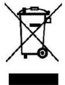
The symbol on the product, or on the documents accompanying the product, the Crossed-Out Wheelie Bin, indicates that this appliance may not be treated as household waste. Instead it shall be handed over to the applicable collection point for the recycling of electrical and electronic equipment, or, if you are buying an equivalent product, to the retailer of the new product.
