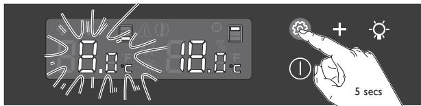
2 Press the **+** or **-** keys to set the temperature of the lower part of the cabinet.
