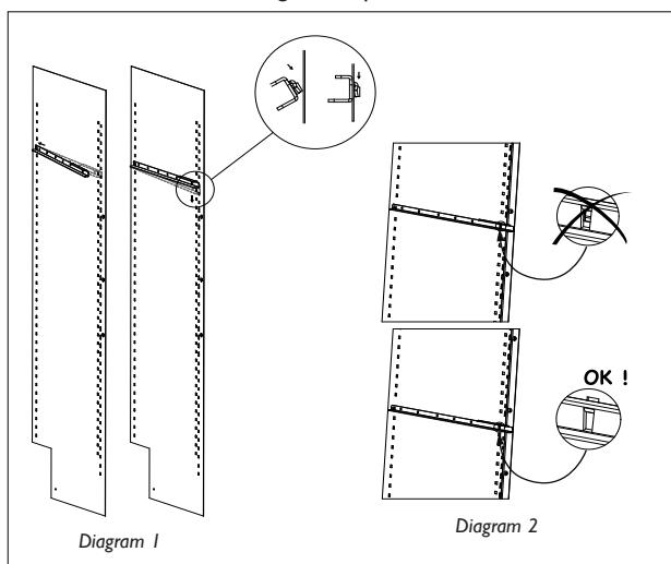
1 Insert 2 guides in the shelf support strips provided. For each shelf, position a guide on the right and a guide on the left (see diagram 1). Ensure that you securely clip the guides into their slot (see diagram 2).
