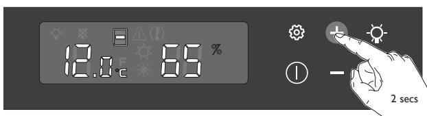
To display the humidity level inside your cabinet, press and hold down the **+** button for 2 seconds
