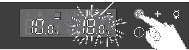
4 Press the **+** or **-** keys to set the temperature of the upper part of the cabinet.
