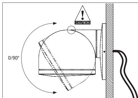
Tighten the two screws on the sides of the speaker to secure Dome on its wall mount.
