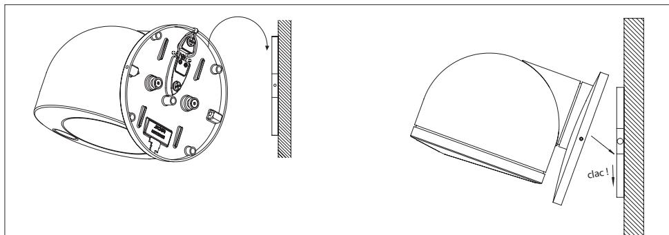
Position the Dome speaker against the wall bracket and then lower it, clicking it into place.
