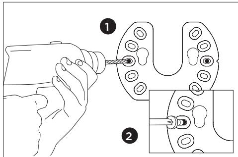
Using the wall mounting provided, mark the 2 fixing holes. Drill these and then insert the wall plugs into the wall. Fix the wall bracket.
