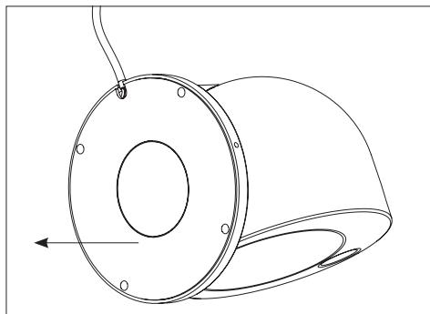
Remove the cover under the base of the Dôme speaker, then connect the cables to the satellite speaker (taking care to observe the correct polarity).
