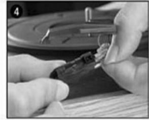
take off the audio-line from the cartridges completely.
