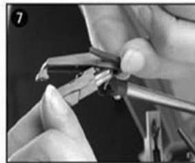
separate the cartridge from the socket lightly.
