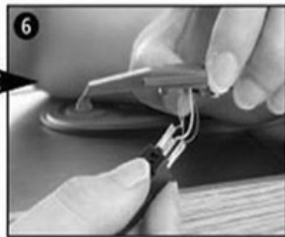
take off cap of the cartridge to expose the needle out.
