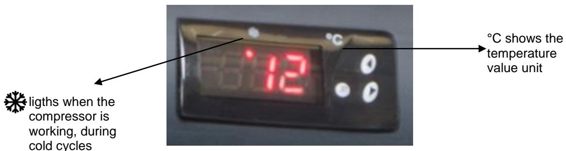
The temperature range can be set as low as 5°C or as high as 18°C to suit your specific storage requirements. The acclimation temperature setting is 12°C.
