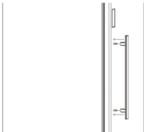
Step 3: after handle is fixed onto the handle screw, there are two hexagon screws popping out, use a hexagon screw driver to fix the screws as below photo:
