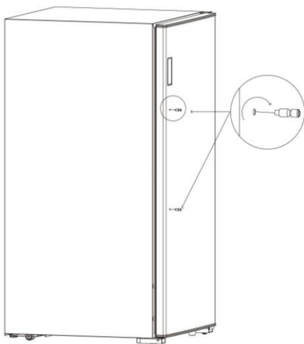
Step 2: there are two holes on the handle base, fix the handle screw into the handle hole at the bottom of the handle base as explained on the drawing here below:
