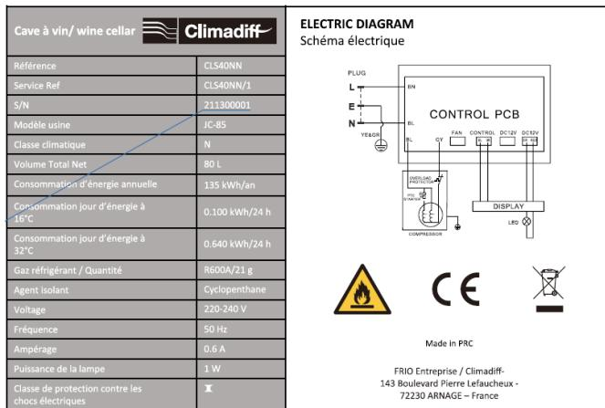
The nameplate attached to the inside or rear of the appliance (depending on the model) includes the entire information specific to your appliance.
