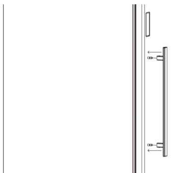
Step 3: after handle is fixed onto the handle screw, there are two hexagon screws popping out, use a hexagon screw driver to fix the screws as below photo:
