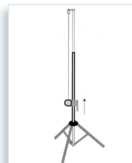
7 - To fold the screen, lift the handle and proceed in reverse order
