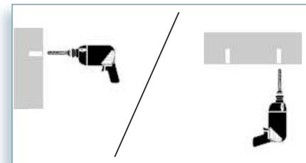
2 - Drill the hole(s) of 5mm diameter
