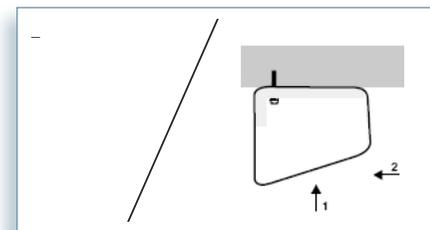
4 - For ceiling mounting, place the screen on the screw using the big holes
