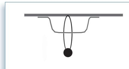
6 - Put the rope with the ball in the central hook of the weighing bar
