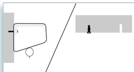
3 - Place plugs in the hole(s) and screw the screen in the wall or place the screw in the ceiling
