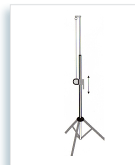
6 - Locate the handle at the required height
