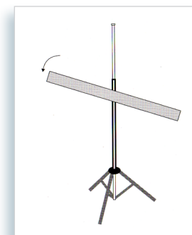
3 - Swivel the screen to its horizontal position
