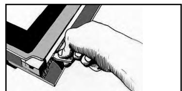
Remove the frame and the glass. Remove all the door's interior windows by rotating them.
