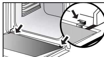
You can dismantle the "SENSOR" plate indicating the presence of a humidity sensor linked to the CHEF mode as it is not essential for operation. Use the plastic wedge supplied to dismantle the door glass.
