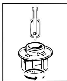
You can replace the bulb yourself. Unscrew the view port and remove the bulb (use a rubber glove, which will make it easier to remove). Insert the new bulb and replace the view port.
