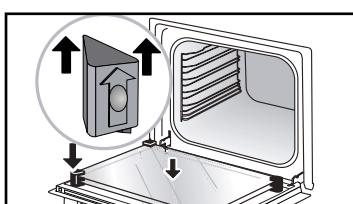
Insert the last glass panel into the metal stops, then clip it in with the side with «PYROLYTIC» facing you and legible.
