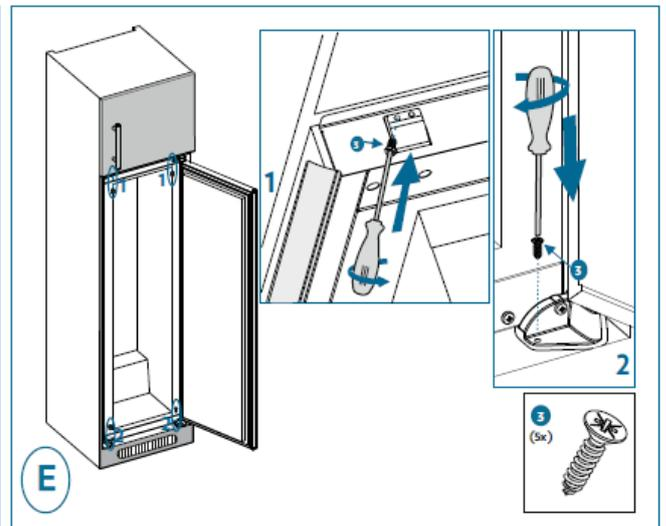
5. Screw a guide into the holes on the appliance side. Insert the sliding rail into the guide and screw it to the door. Unscrew the guide to screw the last screw of the sliding rail to the door. Then attach the sliding rail cover to the sliding rail. Screw the guide back onto the unit by inserting the slide.
