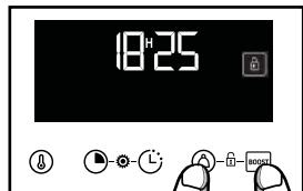
Press and at the same time until the symbol appears on the screen. To unlock, press and at the same time until the symbol disappears off the screen.
