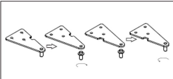
4. Re-fit the door and then upper hinge on left side. Ensure the door is aligned horizontally and vertically, so that the seals are closed on all sides before finally tightening the upper hinge. If necessary, a spanner to tighten the hinge.
