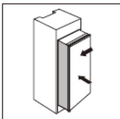
3. Screw a guide to holes in the side of appliance door by short screw. Insert the slider into the guide, then fully open and close appliance door and wooden door to check whether wooden door can close totally and smoothly.
