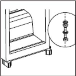
3. Unscrew top hinge pin from the hinge. Then turn the hinge over and screw hinge pin.
