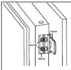
4. Open appliance door and wooden door together and mark the position of slider when the slider can function well at all angle during door closes or opens. Take slider out of guide and fix slider with wooden door by two short screws. Then fix slider cover onto the slider.
