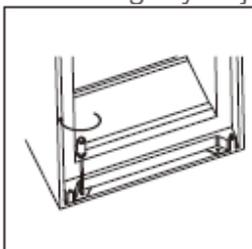
9. Fix top bracket with wooden cabinet by short screws.
