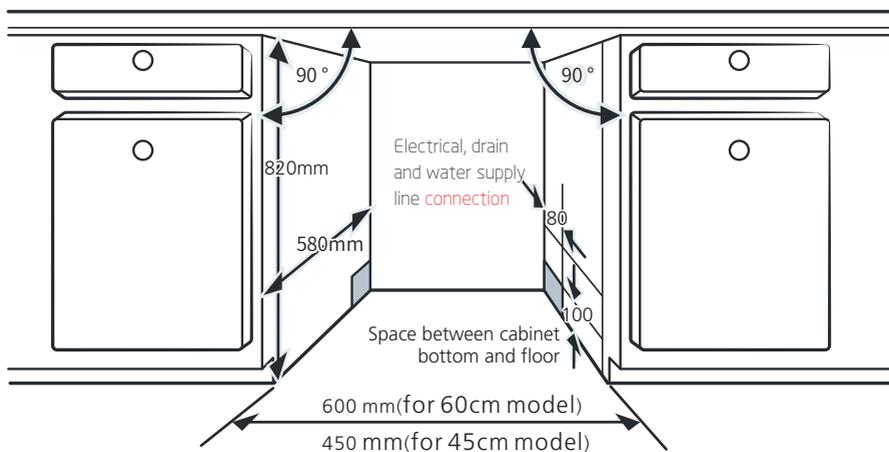
2. If dishwasher is installed at the corner of the cabinet, there should be some space when the door is opened.
