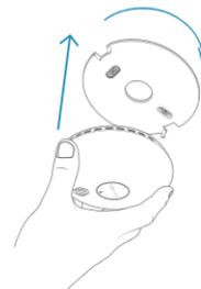
**EN** Then fix the detector to the plate by turning until it locks in place.
