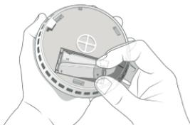
**EN** Fit the batteries in the battery compartment as shown.
