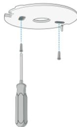
**EN** Fix the plate to the ceiling using the screws provided.
