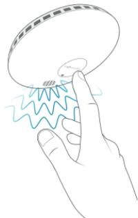
**EN** You should test the smoke detector every month to ensure that it is properly installed and working correctly. You can carry out the test directly on the detector by pressing the central button for three seconds. Note that the alarm will sound for eight seconds. If the alarm does not sound, either the battery is defective or there is another fault (see Troubleshooting on pages 12-13). Do not use a flame due to the risk of damaging the detector.
