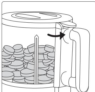
**6.** Turn the locking system (**B**) anti-clockwise to close and lock the lid. The lid is closed properly when the locking system is snapped securely in its slot. You will hear a click, indicating that the blending bowl is ready to be used.
