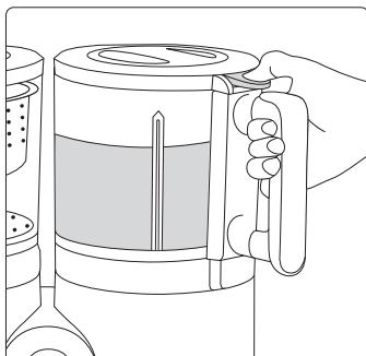
**7.** Press the blending button (**E**) to blend. **ATTENTION:** press the button for short bursts of 5 seconds to prevent overheating. Stop if the blending blade (**D**) spins without any resistance (otherwise, refer to point 15 of the instructions for use).
