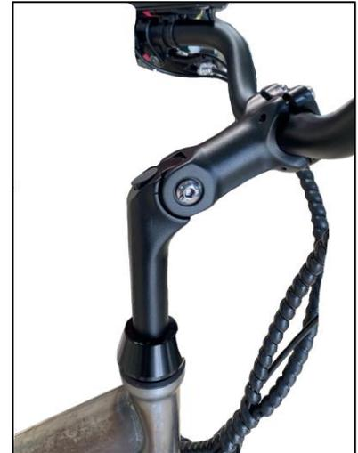
To adjust the tilt of the handlebar, loosen the stem screw-pivot shown in the picture with a 5 mm hex key, select the position and tighten it.
