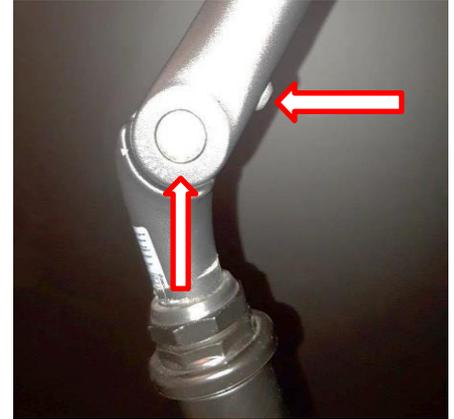
You may then need to adjust the position of the handlebars on the stem by loosening the screws of the stem cover, turn the handlebars at your convenience and tighten these same screws.
