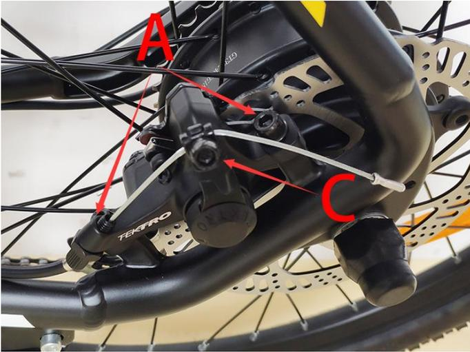
2. When adjusting the brake, please pay attention to brake pad and brake disc (**D point**) for clearance uniformity. Keep vertical and lateral parallel distance, loose the screw to adjust (**A point in the picture**). The brake must be adjusted so that it can be activated by force by 6-8N/m.
