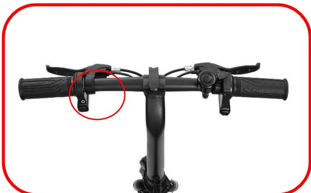
As shown in the photo, the button circled in red allows you to turn your device on and off. Push up to turn on. Then down to turn off.
