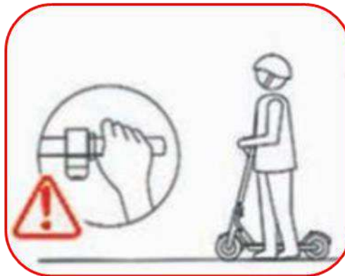
Do not depress the accelerator when you are not on the scooter.
