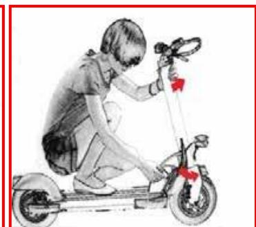
Then return the safety buckle to its original position and make sure your handlebars are stable.
