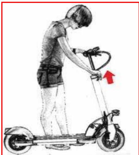
Adjust the size of your handlebars by loosening the clamp buckle on the stem. Be careful not to exceed the height limit indicated. Check that your handlebars are stable and that the clamp is tight.
