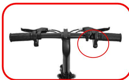
The screen located on the right side of your handlebars allows you to follow the battery level of your device.
