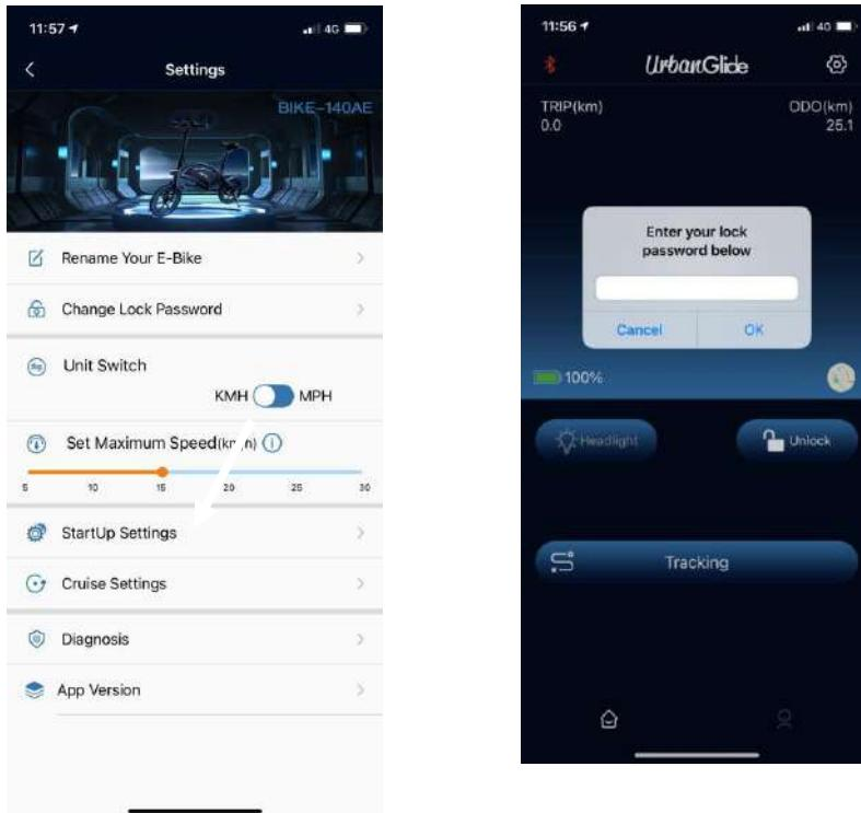
When you click on the lock, the application asks you for a password to lock or unlock your electric bike. When you turn off your bike, it locks automatically, you can ride with it only when it is turned on.
