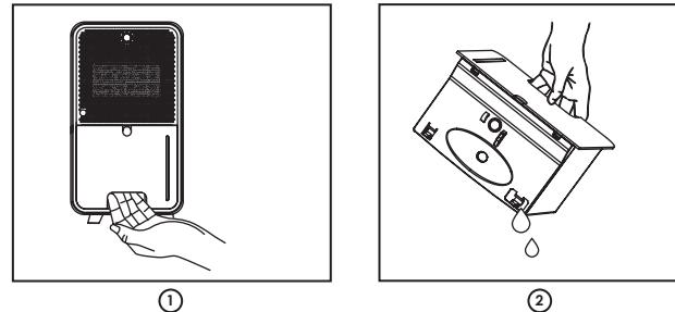
DRAINAGE CONTINU/CONTINUOUS DRAINAGE/KONTINUIERLICHE ENTWÄSSERUNG/DRENAGE CONTINUO/DRENAGEM CONTÍNUA/CONTINUE AFVOER/TRYB: CIĄGŁE OSUSZANIE/JATKUVA TYHJENNYS
