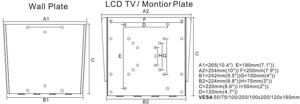
Use the 2<sup>1</sup>/<sub>4</sub>" wood screws, mount the wall plate to wall stud or use enclosed sheet rock mollies
