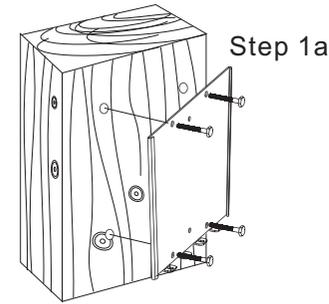
Using the 2<sup>1</sup>/<sub>4</sub>" wood screws, mount the wall plate to **wall stud**
