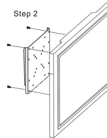
Using the 1<sup>1</sup>/<sub>2</sub>" bolts, mount the monitor plate to back monitor, Depending on your monitor, Use the 75mm or 100mm pre-drilled holes
