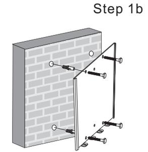
Pre-drill these mounting holes with a 10mm masonry bit to an least 60mm in depth. Using the 2<sup>1</sup>/<sub>4</sub>" wood screws and concrete anchor mount the wall plate to **wall**
