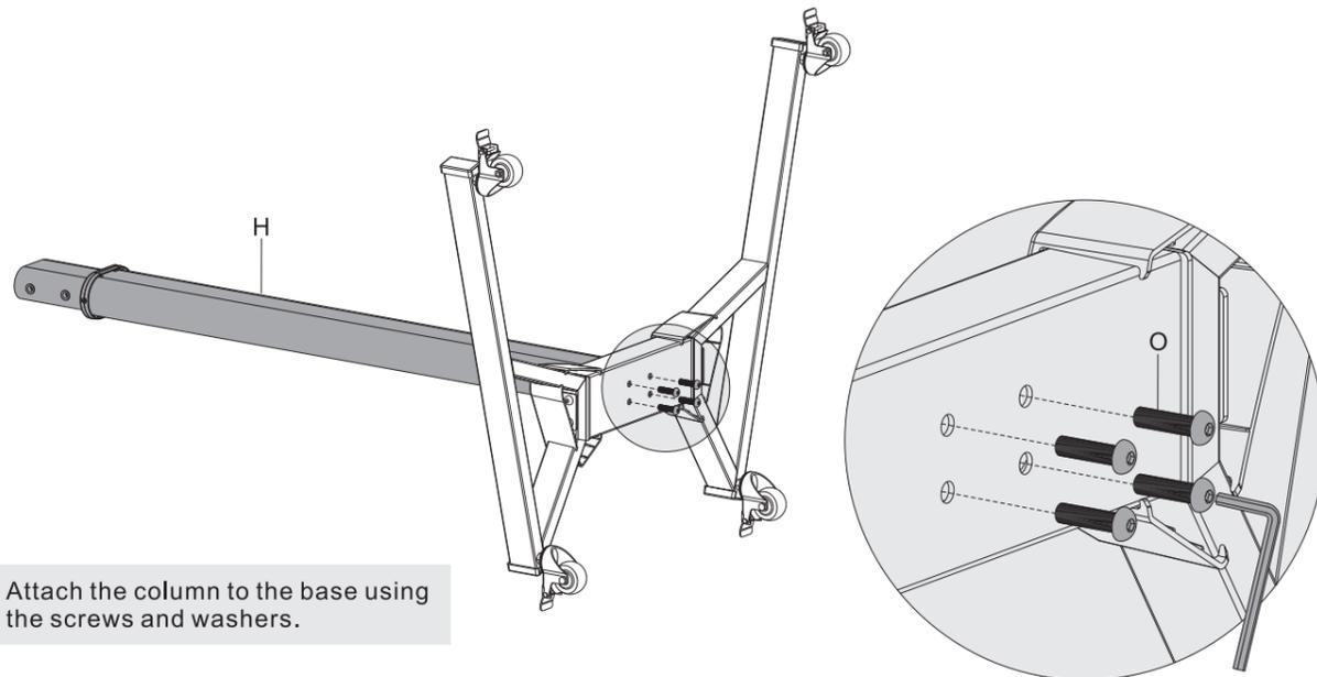
Attach the column to the base using the screws and washers.
