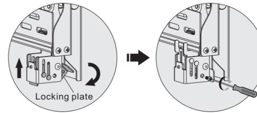
Turn the locking plates downward to fasten the wall plate and tighten the screws to secure.
