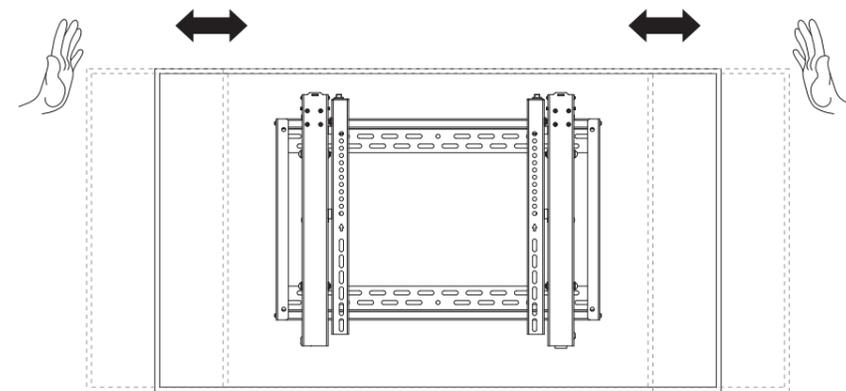
Push the display to left or right to enable fast alignment.
