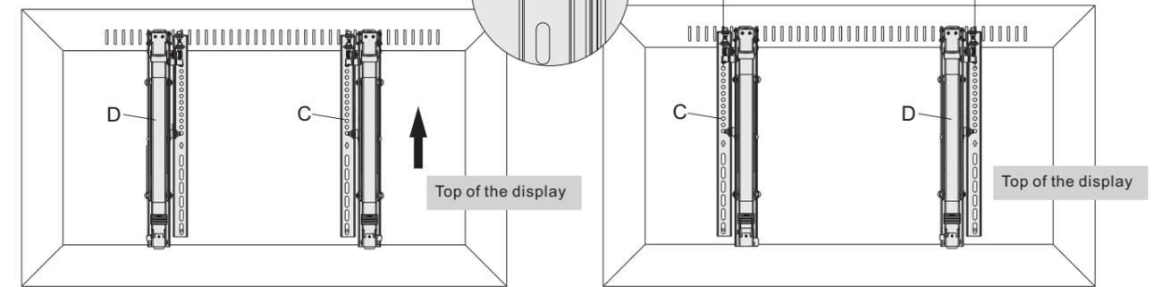
For VESA 600x400, the positions of "D" and "C" are exchanged.
