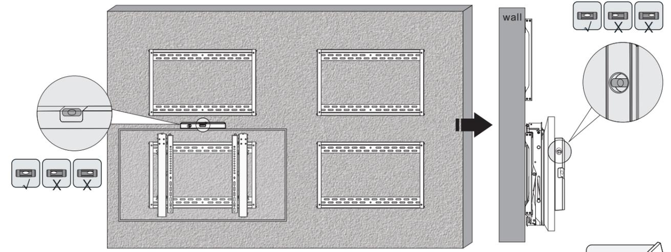
Adjust the display to keep level in vertical and horizontal directions.
