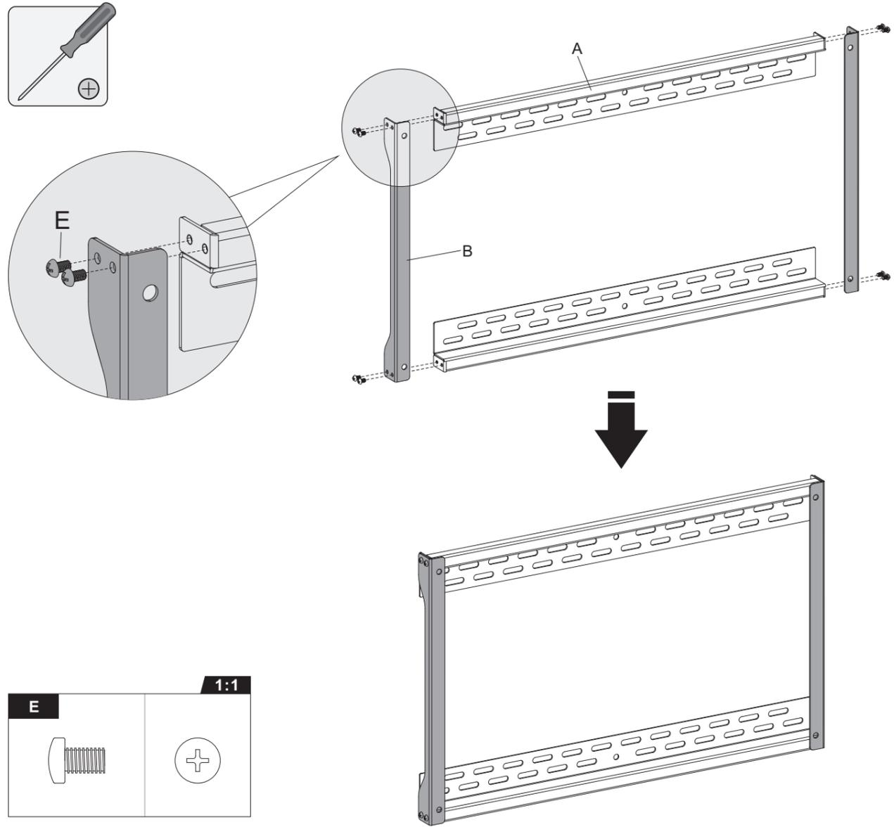
Attach the connecting plates to the wall plates using the appropriate screws.
