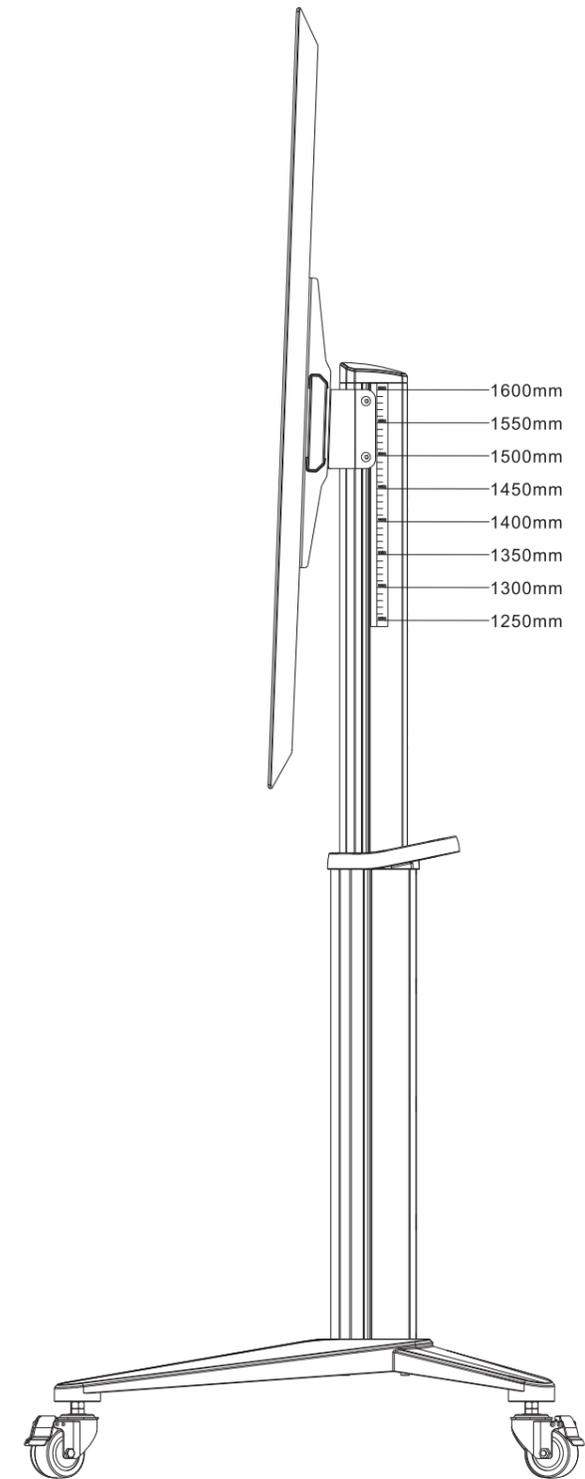
Height markings represent the distance from the floor to the center of the TV screen.
