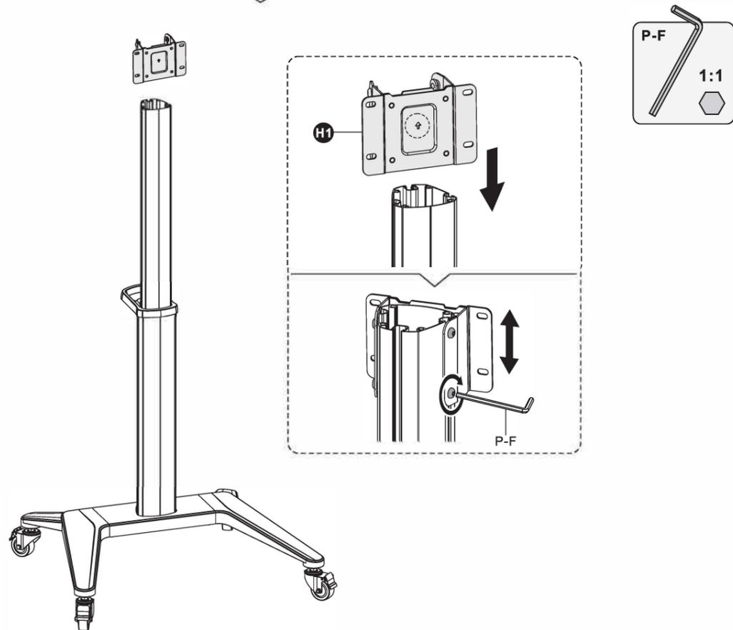
**4. Attach TV Bracket to the Mounting Plate / Fixer les supports TV à la plaque de montage**
